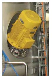
The stator is fixed and will not draw the liquid to circulate. This benefit also allows you to avoid tank baffles.
